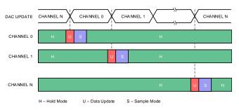
Figure 2. Timing Diagram of the Refresh Cycle
