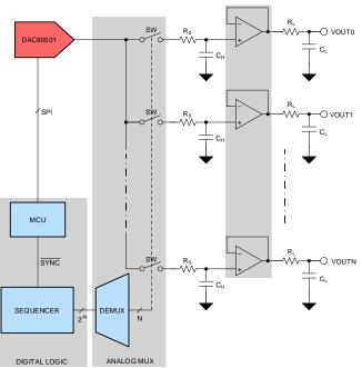
Figure 1. Block Diagram of Multichannel DAC using S&H
